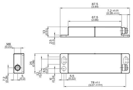
The actuators have the same dimensions as the sensors, but without plug connector.
