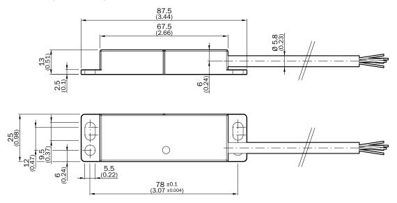
The actuators have the same dimensions as the sensors, but without connecting cable.
