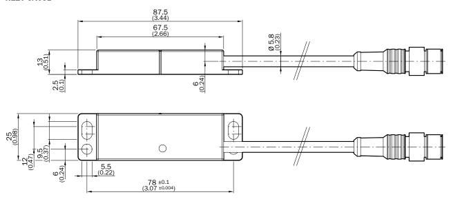
The actuators have the same dimensions as the sensors, but without connecting cable.
