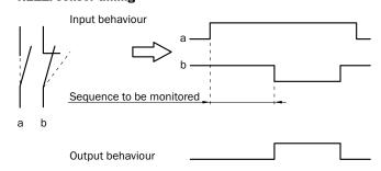
Both contacts must change output state, before it can be reset. Compliance with this sequence must be monitored by the safe evaluation unit.
