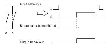
Both contacts must change output state, before it can be reset. Compliance with this sequence must be monitored by the safe evaluation unit.
