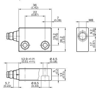
The actuators have the same dimensions as the sensors, but without plug connector.
