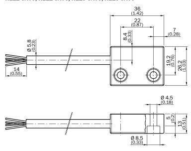
The actuators have the same dimensions as the sensors, but without connecting cable.
